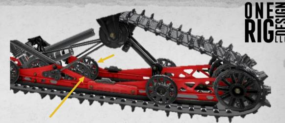
Step 2: Using 10 mm wrenches remove bogie inside bogie wheels marked above.
