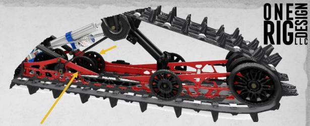
Step 2: Using 10 mm wrenches remove bogie inside bogie wheels marked above.
